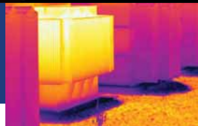
Transformer Thermal Image
