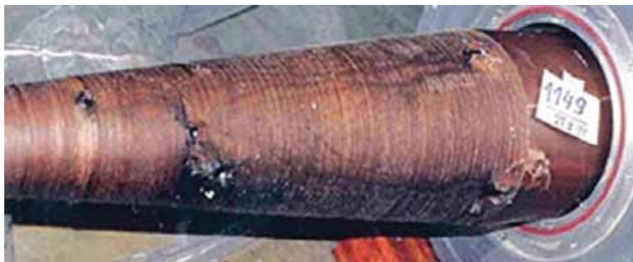
Figure 2: Moisture Contamination in Oil End Part of Bushing
