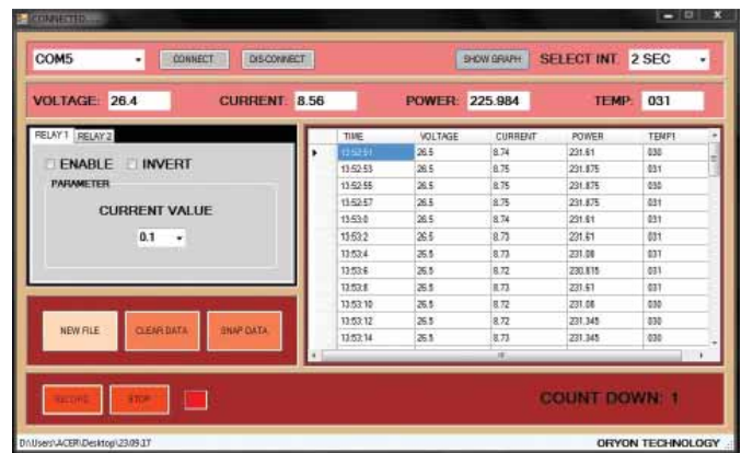
Figure 4: Data logger recording and displaying solar panel data as numeric values
