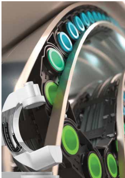
The lokchain principle: automatically extending pins (blue) hold the lokchain firmly in the guide trough. When the chain link bends into the radius, the pin retracts automatically (green) and releases the chain. Due to its flexibility, the e-chain can be used for example in a rotating C-arm X-ray device.
