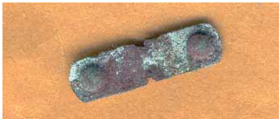
Chlorine corrosion of Contact following PVC fire
