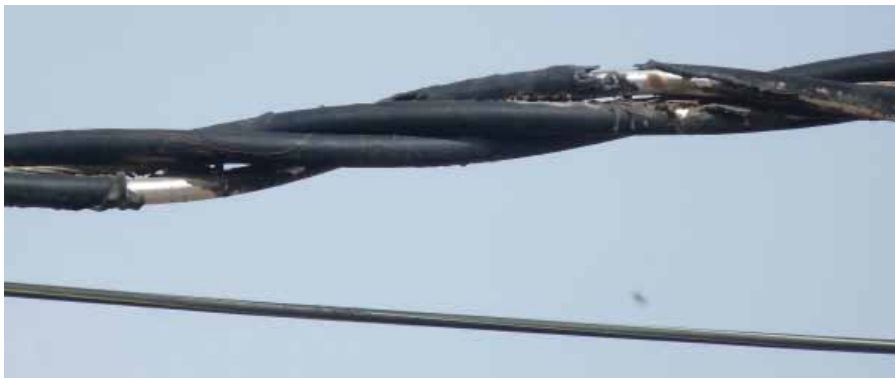
11 KV AB Cable damaged due to sparking between cores
