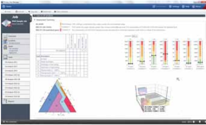
Picture 2: The PTM software assesses DGA results using interpretation methods such as Duval's triangles or gas ratio methods according to IEEE C57.104 and IEC60599
