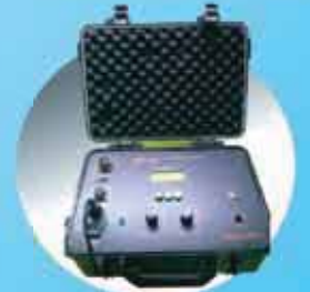
Auto. Transformer Ratio Meter
