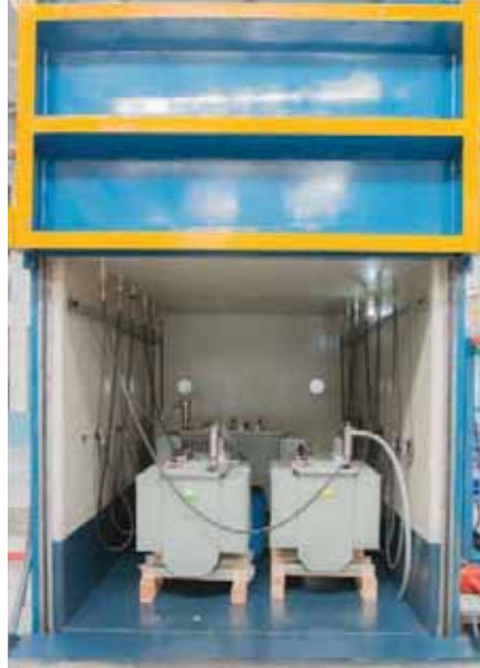
Oil filling in totally controlled atmosphere in a vacuum condition...
