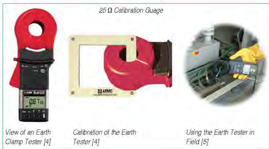
Fig. 3: Earth Clamp Tester and its usage
