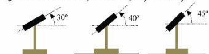
Fig. 3: Inclination of the PV panels installed at UIET, Panjab University
