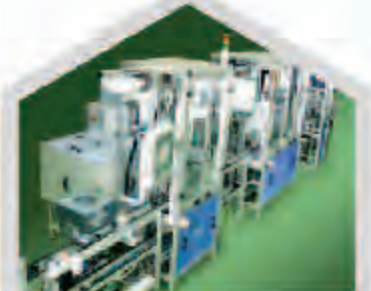
Contactor Assembly Lines
