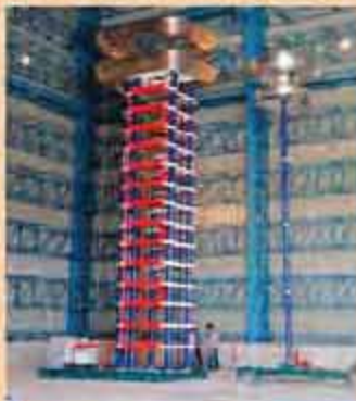
2400kV, 240kL impulse Voltage Generator
