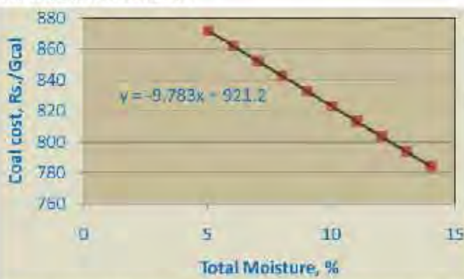
Fig. 15: Sensitivity of Indian coal price (Rs./Gcal) to total moisture if moisture effect is considered
