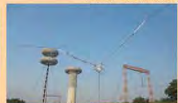
1200kV Insulator String testing
