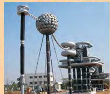
1200kV CYT under test
