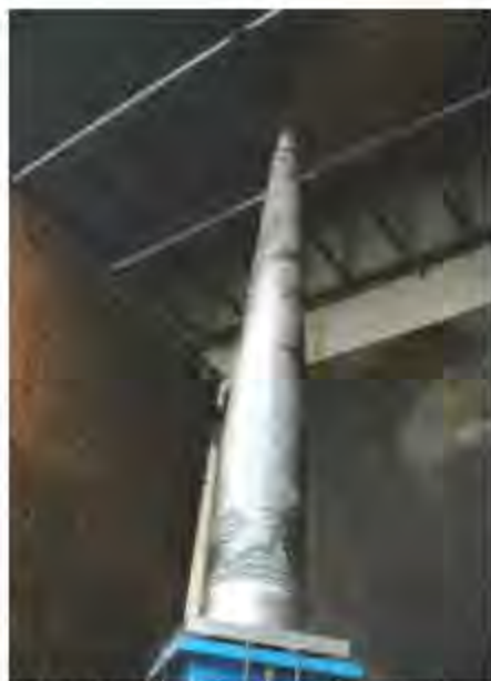
Fig. 6: 420 kV outdoor termination after the power arc test
