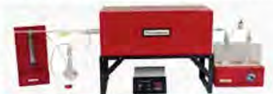
Fig. 1: Test set-up for determining Halogen Acid by titration (IEC 754-1)
