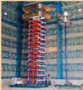
2400kV, 240kV Impulse Voltage Generator
