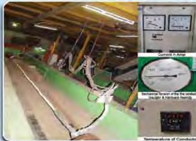
Testing of HTLS Conductor with Dead-End Assembly
