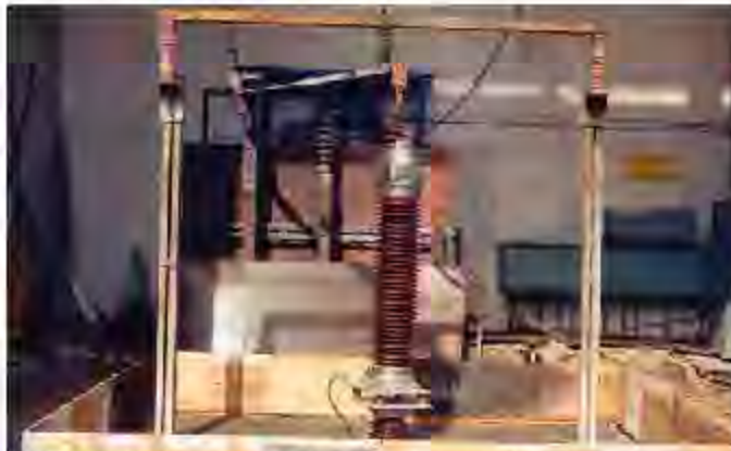
Fig. 5: 120kV porcelain clad surge arrester before test
