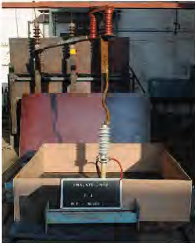
Fig. 7: The photograph of polymer surge arrester before test
