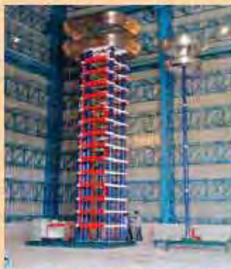
2400kV, 240kJ Impulse Voltage Generator
