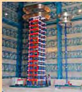
2400kV, 240kJ Impulse Voltage Generator
