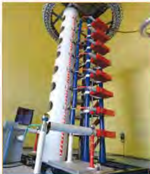
1800 Kvp, 80 kJ Impulse Voltage Generator
