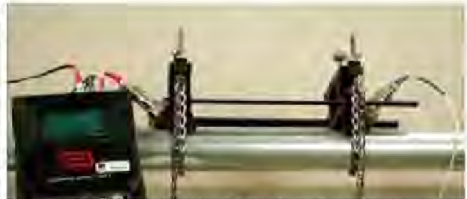
Ultrasonic Probes Installed on Piping for Velocity Measurement...
