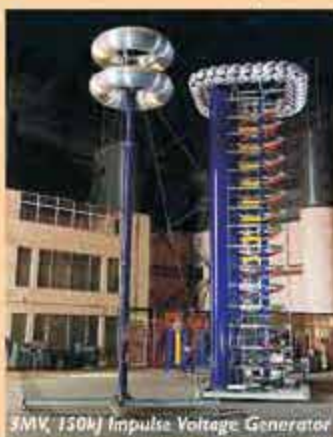
3MV, 130kJ Impulse Voltage Generator
