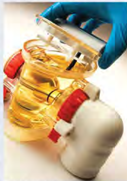
Fig. 3: Correct fitting of the baffle plate is essential...
