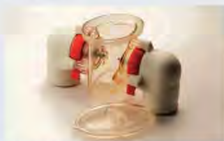
Fig. 1: A typical modern test vessel assembly fabricated from shatter resistant materials...
