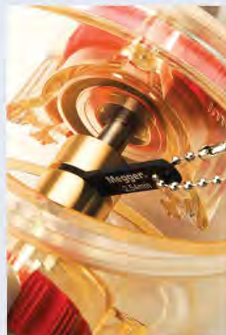
Fig. 2: Using a gap gauge to set the electrode spacing...
