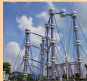
HVDC Generator at UHVRL, Hyderabad
