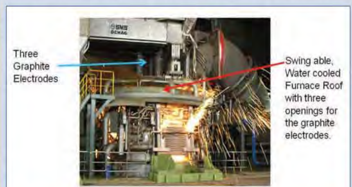
Fig. 2: Actual Electric Arc Furnace in operation
