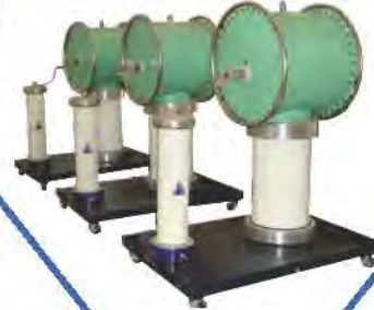
Transformer Loss Measuring System
