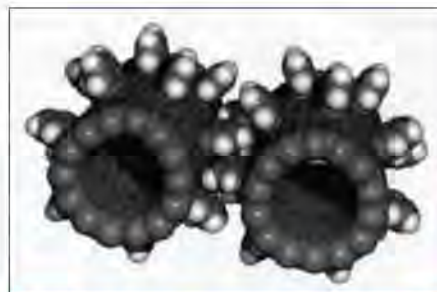
Fig. 4: These nanogears were made by attaching benzene molecules (outer white blobs) to the outsides of carbon nanotubes (inner gray rings). By courtesy of Great Images in NASA
