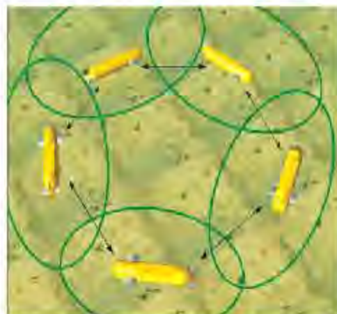
Fig. 4: Formation controls of multiple AUVs using predefined shape
