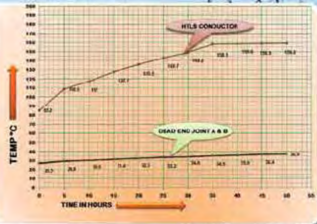
Testing of HTLS Conductor with Dead-End Assembly
