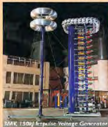
3MV, 150kJ Impulse Voltage Generator
