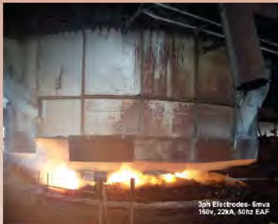
Fig. 1: 6.5T, 6mva, 3Ph, EAF at its normal operation
