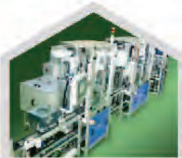
Contactor Assembly Lines
