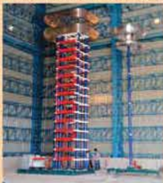
2400kV, 240kA Impulse Voltage Generator
