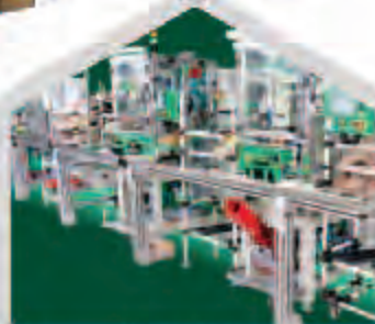
MCB, MCCB Assembly Line
