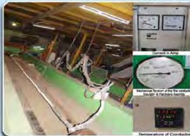
Testing of HTLS Conductor with Dead-End Assembly
