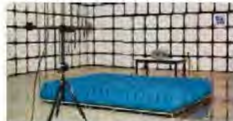
10 Meter Semi - Anechoic Chamber for EMI-EMC Test
