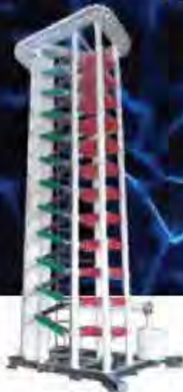
Impulse Voltage Test System
