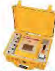
Winding Resistance Meter
