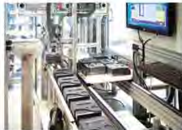
The new automatic assembly lines for smart meters in CG's ZIV facility in Spain...
