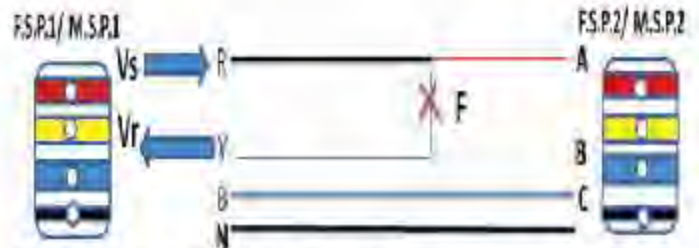
Fig. 2: Short circuit fault locating principle
