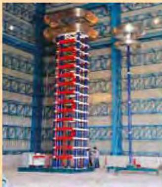
2400kV, 240kJ Impulse Voltage Generator
