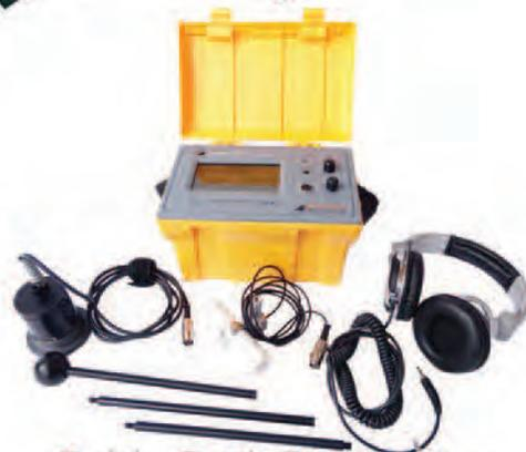
Cable Fault Pin pointer
