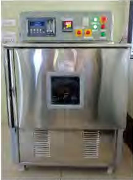
Fig. 1: Programmable ozone test chamber...
