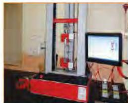
Automatic Universal Testing Machine with Extensometer
