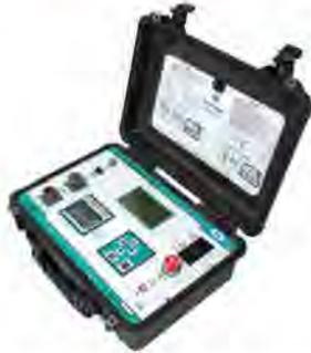
Motwane has launched a new transformer turns ratio meter XTRM-3, which is a new generation, fully automatic transformer turns ratio tester. It measures the transformation ratio of single phase and three phase transformers using modern electronic techniques. It is a micro controller operated, user friendly and reliable tester.
