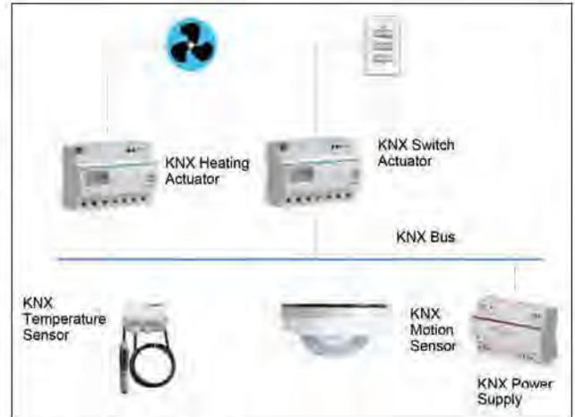
Fig. 2: Typical KNX Network...
