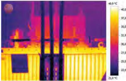
Depending on the type of insulation, the connections, cores or insulation in components of medium-voltage installations such as transformers can be inspected for thermal irregularities.
