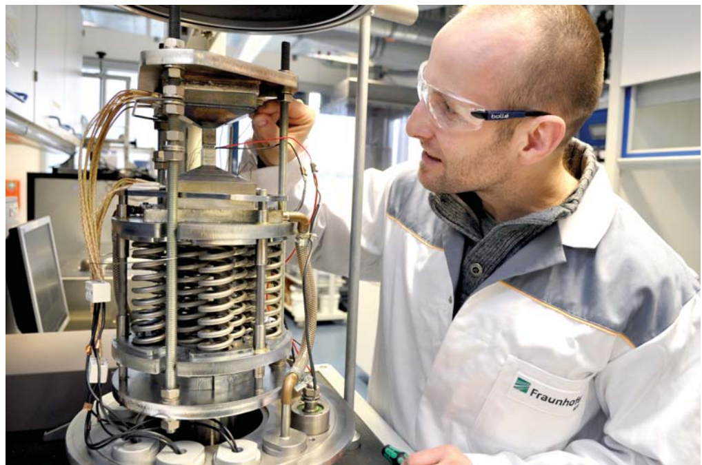
Test stand for efficient and autonomous power generation of the waste heat of an all-ceramic heating conductor working at 800 °C in ceramic TEG modules...
