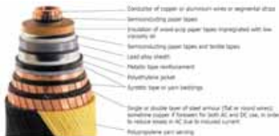
Fig 2. Oil Filled Paper insulated Cable...
