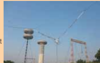
1200kV Insulator String testing
