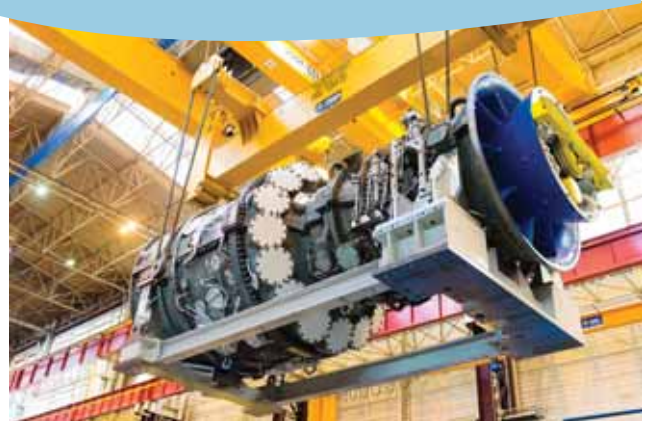
The fully assembled 9HA gas turbine being transferred for packing and shipping...
