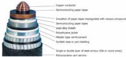
Fig 1. Mass Impregnated, Paper insulated Cable...
