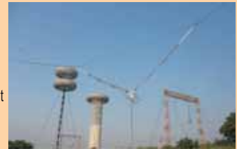
1200kV Insulator String testing
