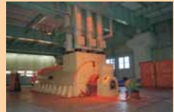
2500MVA Short Circuit Generator
