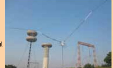
1200kV Insulator String testing
