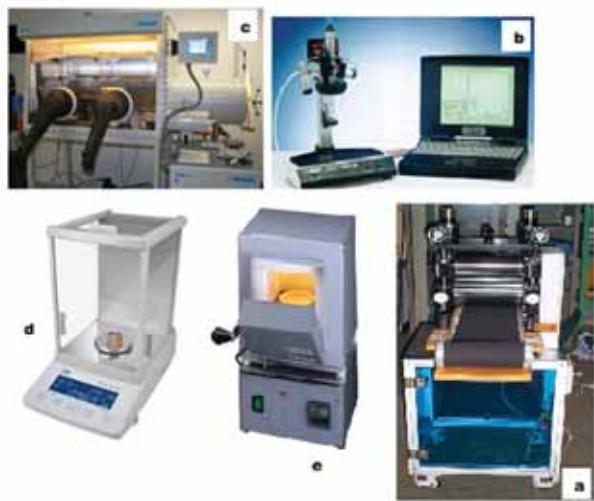
Figure 4: Some of the instruments required for supercapacitor research. Anticlockwise from the top (a) Calendaring machine (b) Cyclic Voltammeter (c) Glove box (d) High Precision Electronic balance (e) Muffle Furnace...
