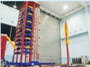
1200 Kv Impulse Voltage Generator
