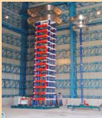
2400kV, 240kJ Impulse Voltage Generator
