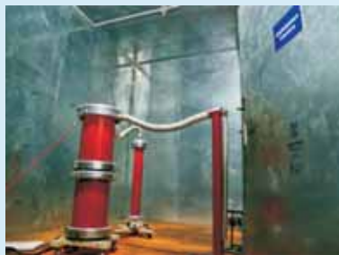
Partial Discharge Test
