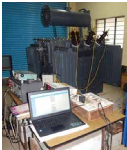
Fig.2: General Test set up for Temperature rise test...
