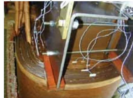
Fig. 4: Location of sensors to predict hot spot temperature...
