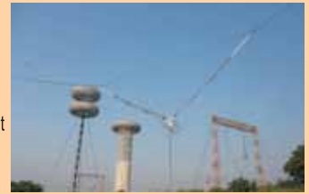
1200kV Insulator String testing
