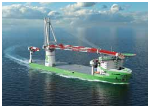
Offshore construction vessel being built for DEME
