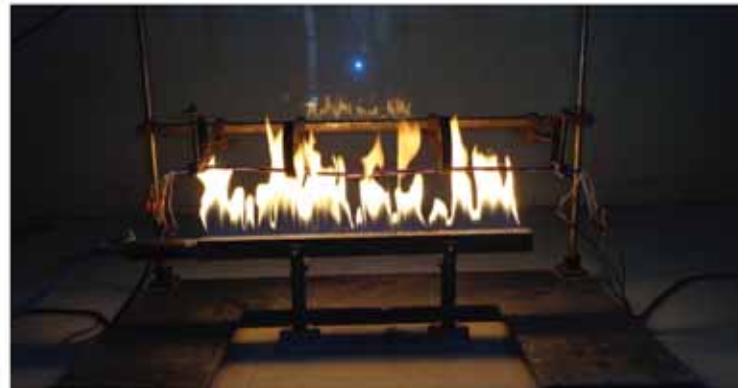
Fire survival – Cat CWZ Set Up
