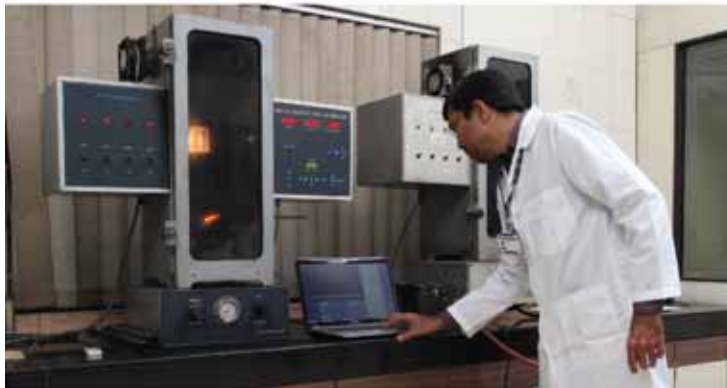
Smoke Density Testing in progress
