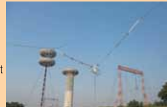
1200kV Insulator String testing
