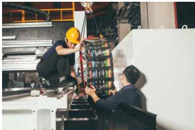
igus energy chains, including cables and mounting frame, are delivered as fully-assembled readychains. The energy supply systems are then fitted within half a day instead of several weeks. (Source: igus GmbH)
