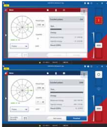
Figure 4: The CMControl P App for Android Tablets and Windows PCs is the easiest way to perform a quick manual meter test.
