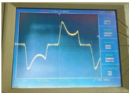
Figure 8: Current Waveform of 60W LED Street Lamp
