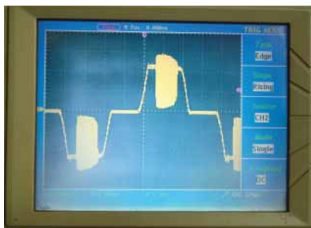
Figure 9: Current Waveform of 200W Flood Light
